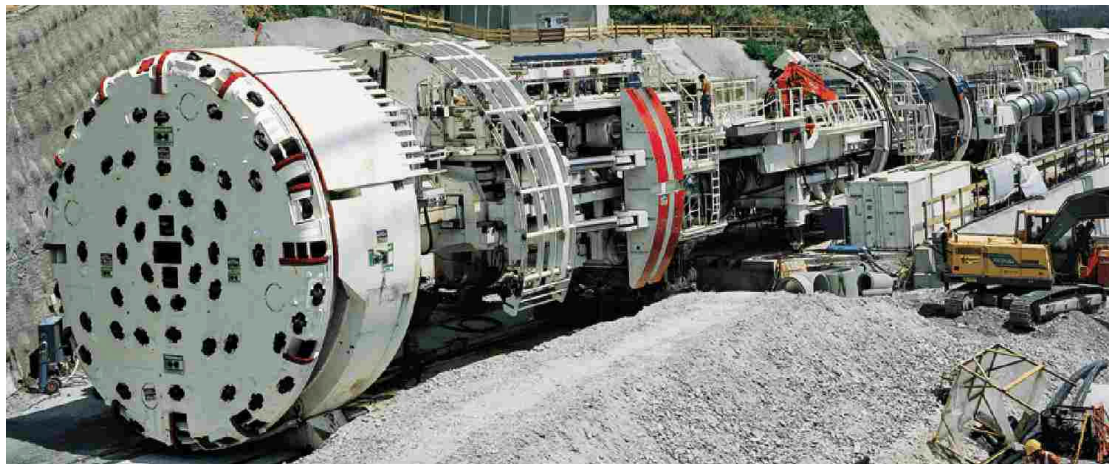
Figure 5 Hard Rock TBM
